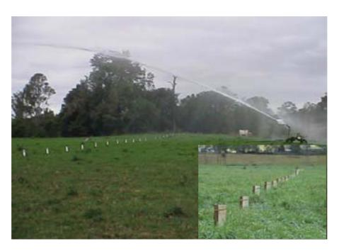
**Figure 5.** Catch cans laid out under a travelling gun irrigator to record the depth of water applied for use in calculating application uniformity (Table 8).
