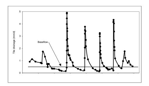
**Figure 13**. Tile drainage flow in furrow irrigated vineyard.
