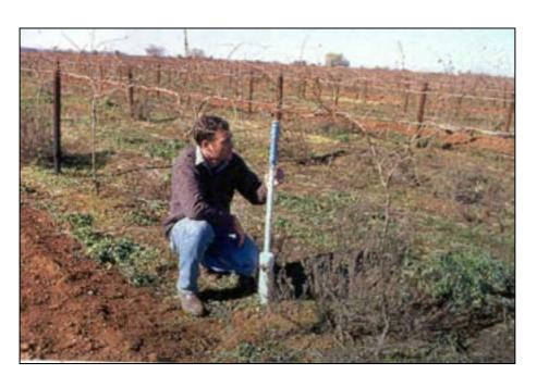
Figure 11. Testwell in vineyard with capacitance logger
