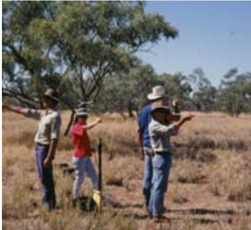
Figure AI4 Rangeland officers estimating tree basal area using the Bitterlich Stick method, at a QGRAZE site, Cloncurry, north-west Queensland.
