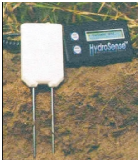
FIGURE 6.19 Campbell 615 water content reflectometer with HydroSense handheld reader.
