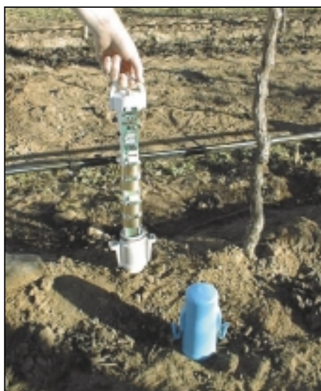
FIGURE 6.10 C-Probe with Adcon telemetry unit.
