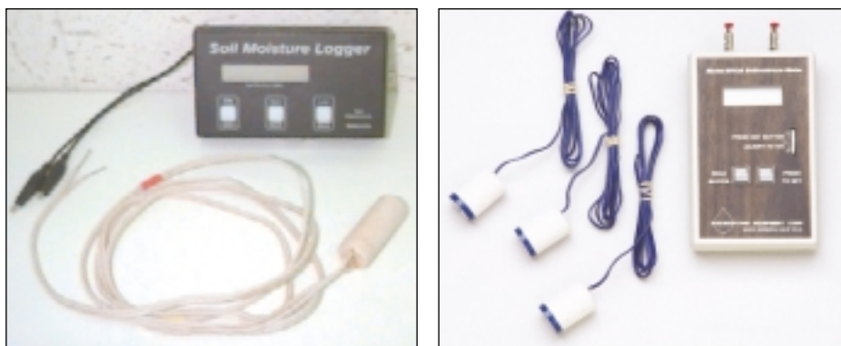
FIGURE 6.3 Gypsum blocks and readers/loggers.
