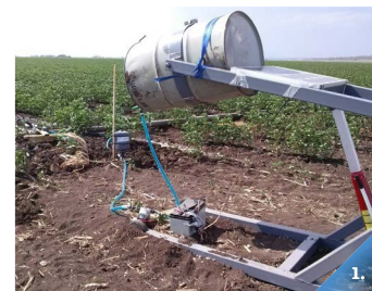
FIG. 1 Fertigation unit for injecting liquid N into gated pipe for field trial.
