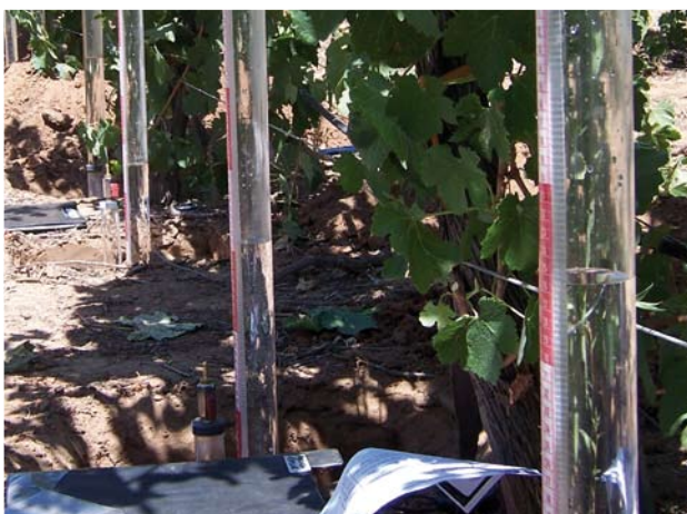
Measuring infiltration in one of the Barossa Valley vineyards being studied by Rob Murray
