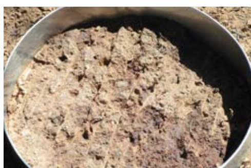
A fracture surface at the boundary of topsoil and subsoil prepared for infiltration measurements; roots and macro-pores are clearly visible.
