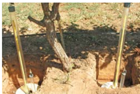
Infiltration measurements under way using disc permeameters
