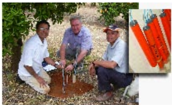
Tapas Biswas (left), from SARDI with Graeme Sanderson (middle) from NSW DPI and Jahangir Alam (right) from SA Rural Solution whilst installing solution extractors (top right) for monitoring salt leaching in a citrus grove at Dareton, NSW
