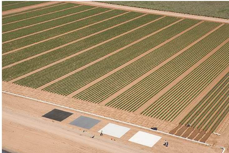
Figure 18: Image of field obtained using aerial photography with reflectance panels to calibrate crop coverage images (French et al. 2011)
