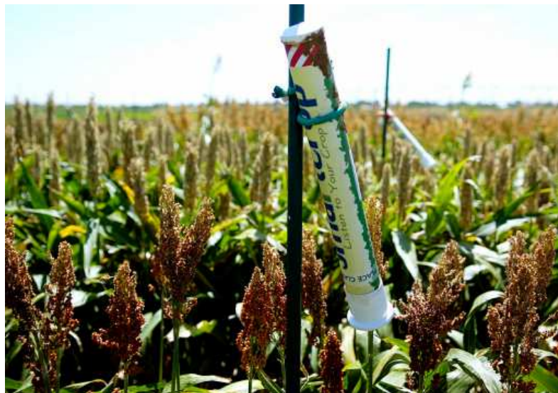
Figure 28: Smart Crop infrared thermometer fixed in sorghum field
