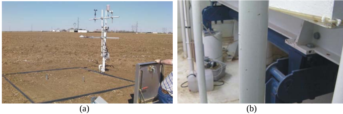
Figure 24: Lysimeter and access at research station in Bushland, Texas
