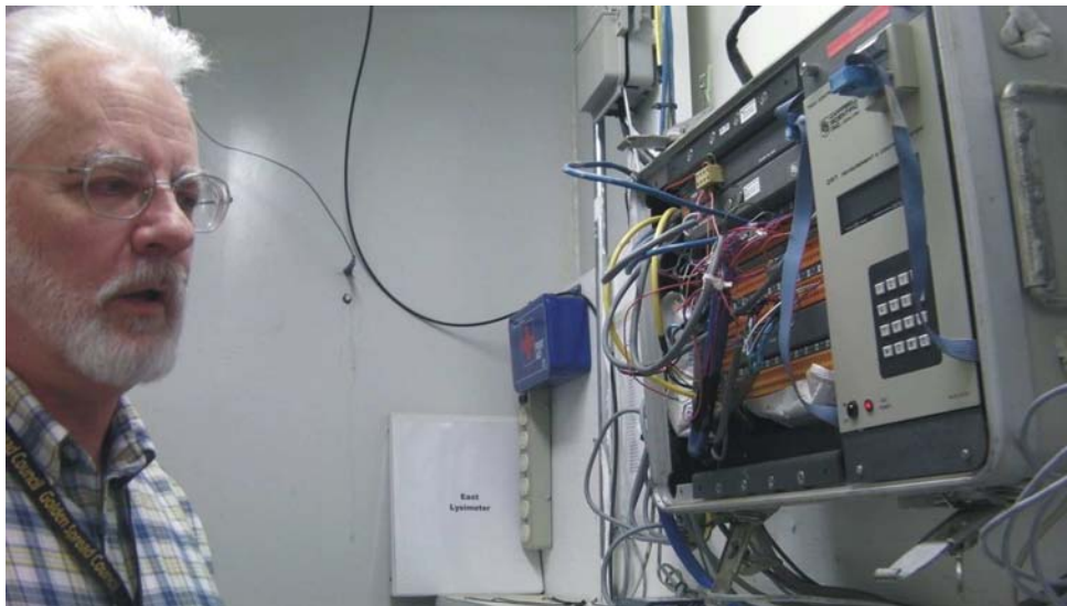
Figure 25: Dr Steven Evett and the lysimeter control panel
