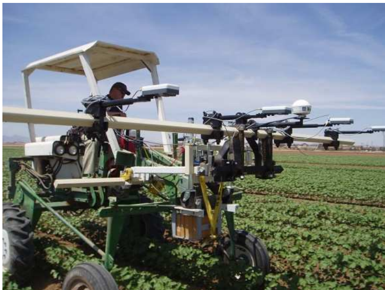
Figure 17: NDVI sensors on tractor for estimation of soil water depletion (French et al. 2011)
