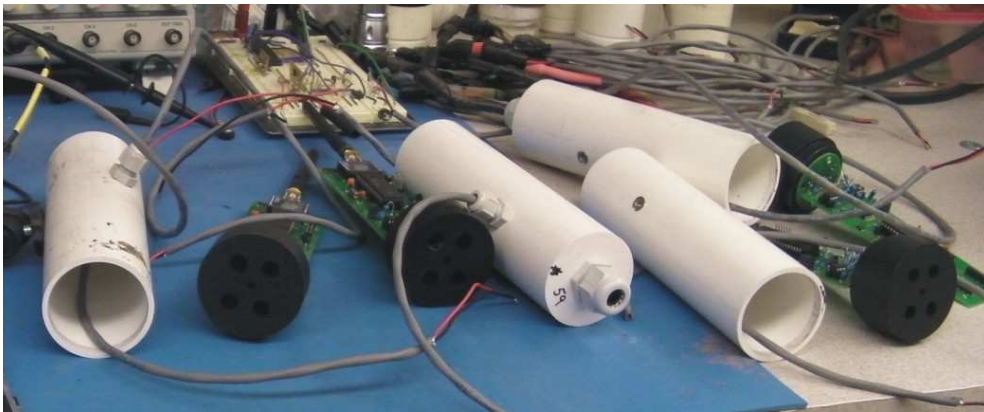
Figure 23: Prototype of infrared thermometer with colour sensor
