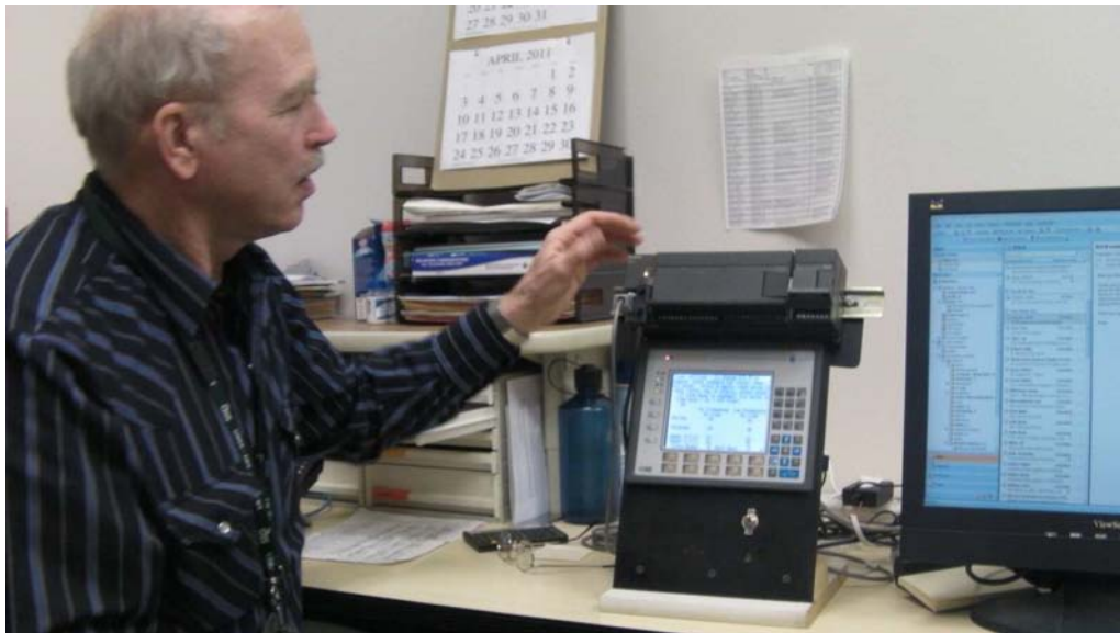
Figure 14: William Eversen explains the programmable logic controller used to control the variable-rate applicators
