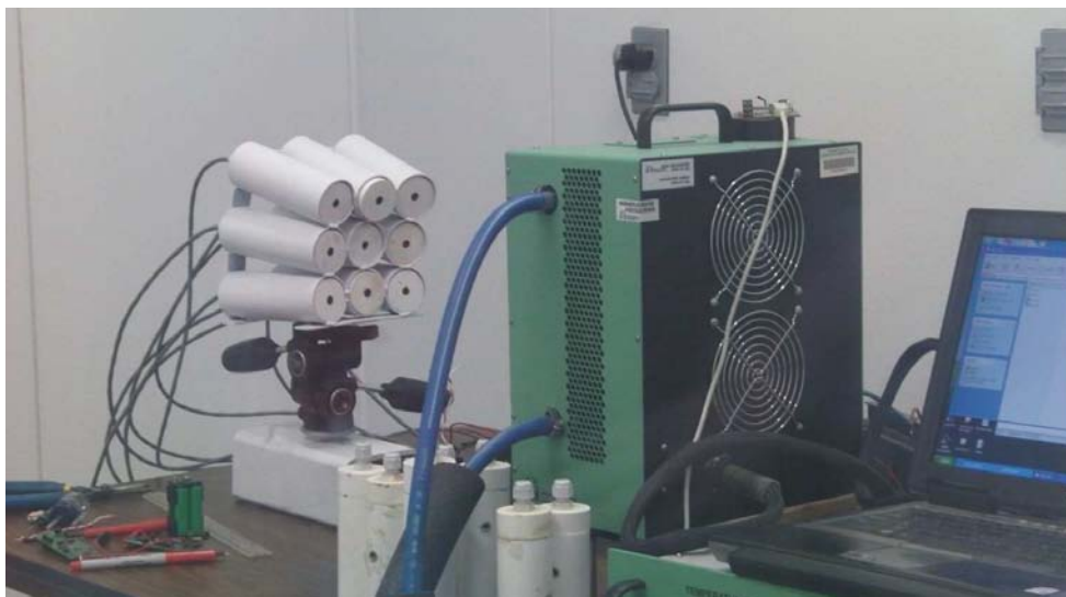
Figure 21: Nine infrared thermometers being calibrated in controlled temperature room
