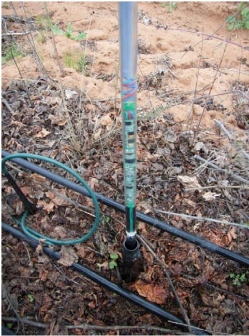
The soon to be commercialised prototype Soil Salt measuring tool developed jointly by Dr Andrew Skinner and Dr Richard Stirzaker using NPSI seed funding. The probe is inserted in the black cylinder to pre-determined soil levels then measures the salt levels which are electronically dumped onto grower computers.
