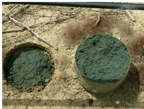
Figure 9. Horizontal distribution of dye tracer after infiltration of 32 mm of rainwater followed by 64 mm of dye solution.
