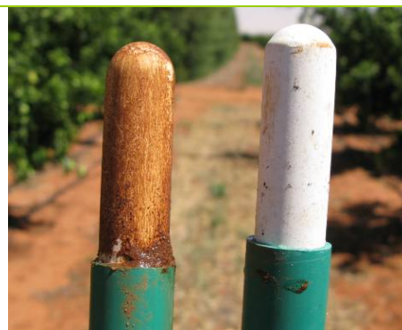
Figure 24 Ceramic cup sampling devices removed from soil in the Atwood navel orange irrigation/fertiliser management trial at Dareton
