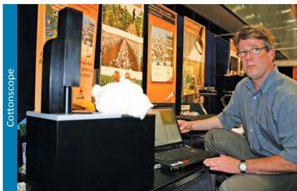
CSIRO Materials Science and Engineering researcher, René van der Sluijs with the newly commercialised Cottonscope instrument that measures fineness and maturity quickly and accurately
