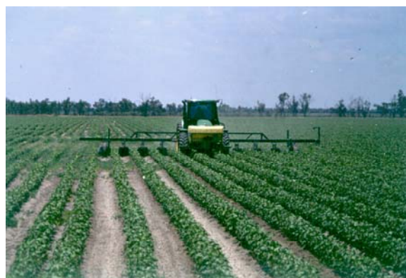
A purpose-built shielded sprayer being used to inter-row spray a troublesome weed, polymeric takeall, in young cotton.
