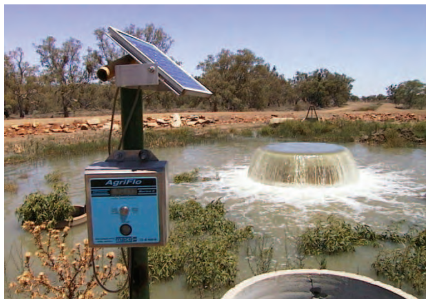
Figure 2.9.1. One of the commercially available water flow meters capable of measuring bulk flows onto and off an individual field
