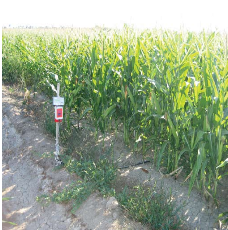
Figure 3a.1.2. A G Bug data logger and wireless retriever (in a maize crop).
