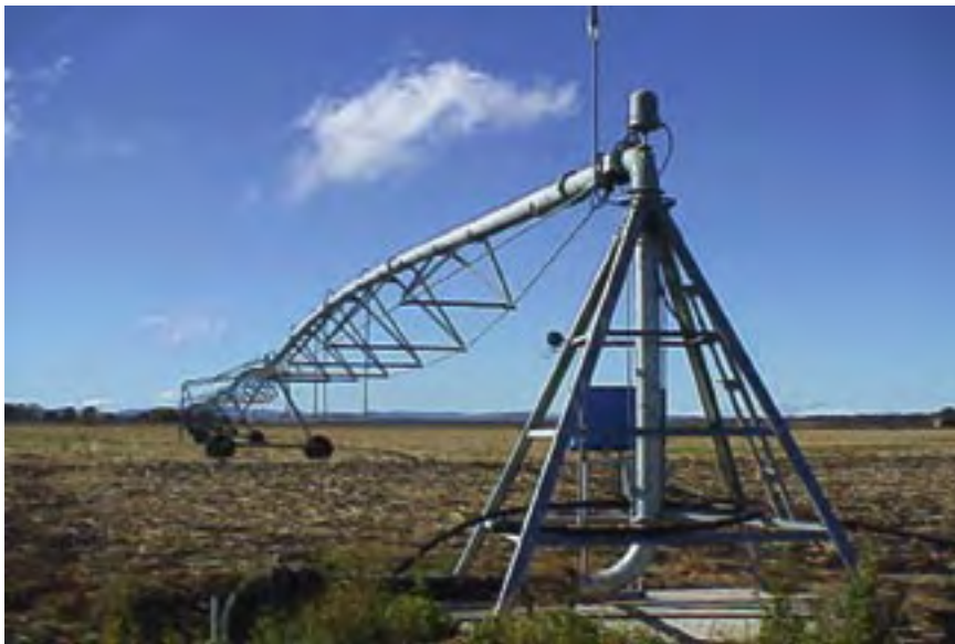
Figure 4.6.1. Centre pivot irrigation machine showing centre tower, spans, and wheel towers
