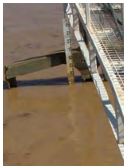
Figure 2.6.3. Gauge board for the storage curve in Figure 2.6.2
