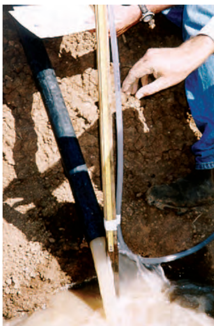
Figure 2.9.3 Measuring head height and using theoretical flow charts to estimate siphon flow rate
