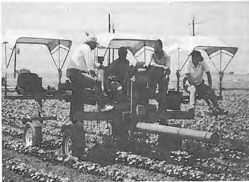
Figure 6. Mobile EM38 salinity assessment module of the U.S. Salinity Laboratory.
