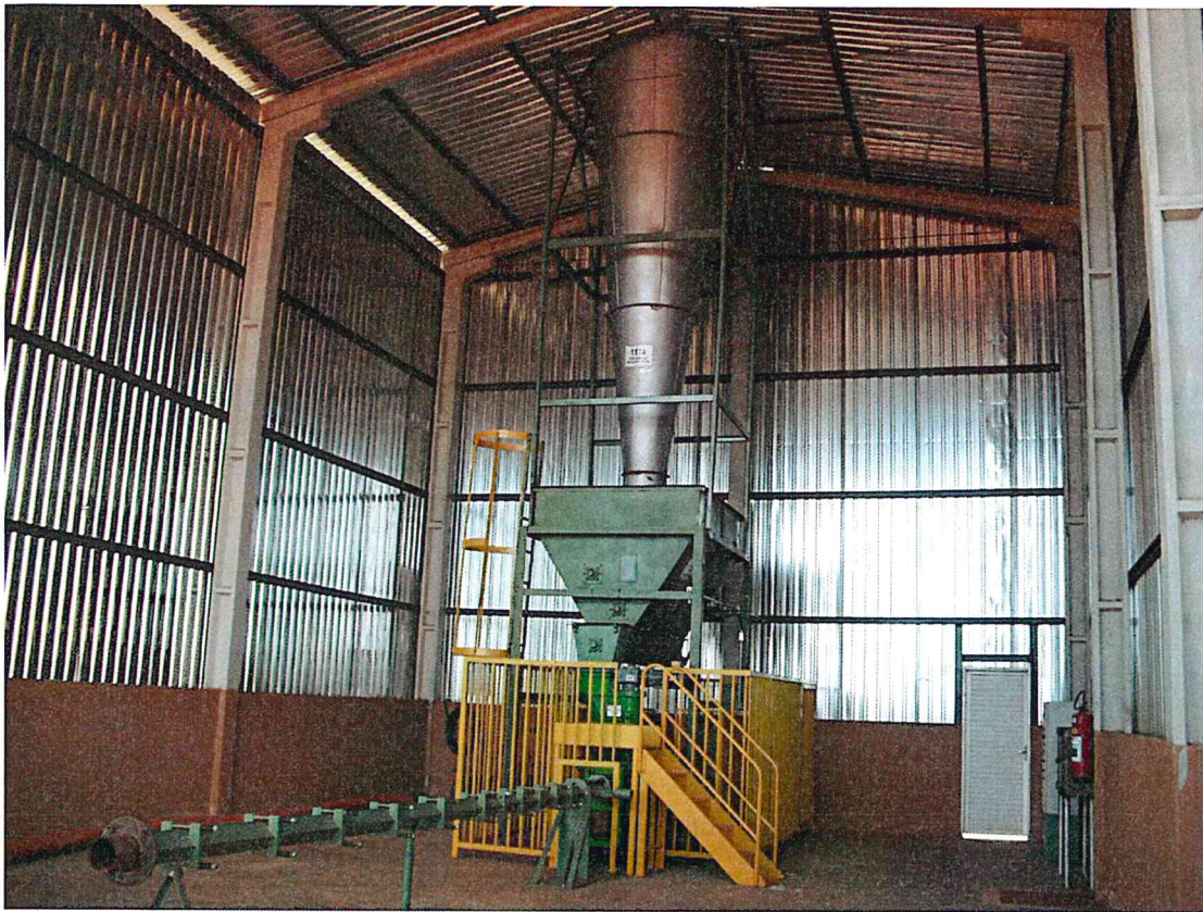
Cotton gin trash being compressed into briquettes for burning
