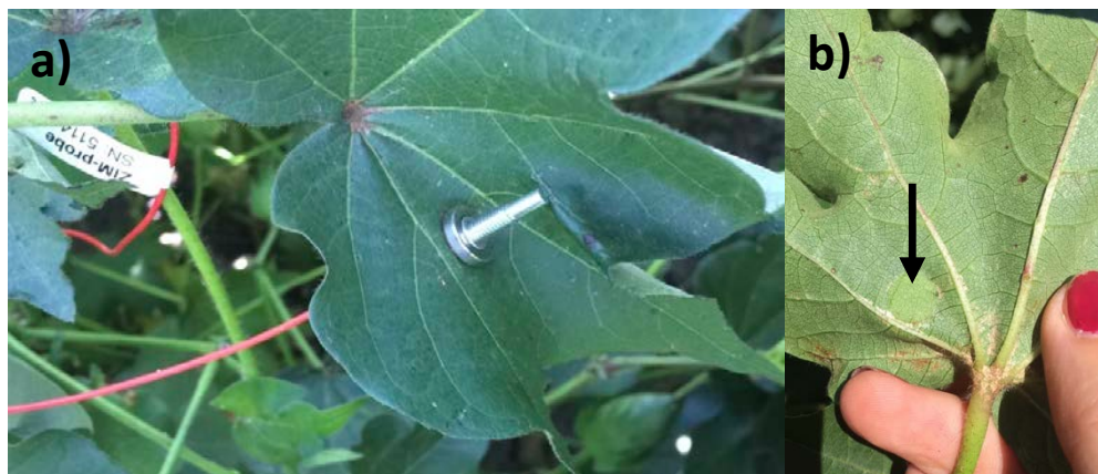
Figure 2. Examples of a ZIM-probe clamped on a cotton plant in the field (a) and leaf patch after removal of the probe (indicated by arrow) at the end of the experiment (b). Note the slight discoloration due to loss of chlorophyll in (b).
