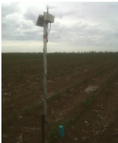
Figure 3: Capacitance probe installed in the experimental field.
