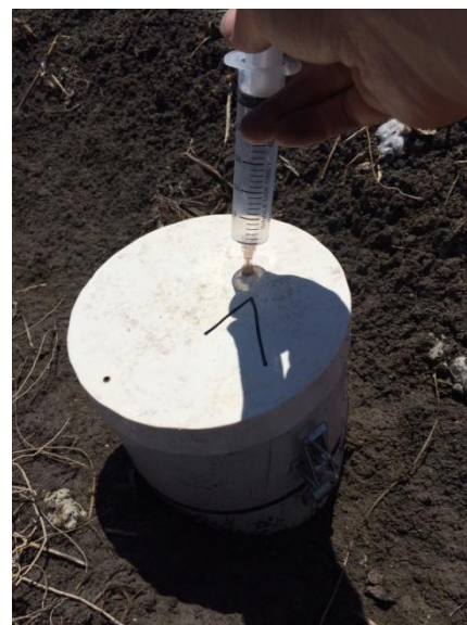
One of the 36 gas chambers in the field, used to collect the nitrous oxide emissions from the soil
