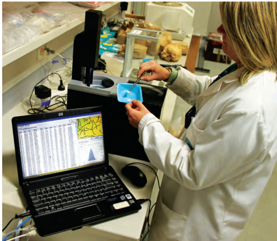
The cotton industry, through CRDC, has invested more than $1 million in the development of SiroMat (measuring fibre maturity) and Cottonscan (assessing fibre fineness) and these technologies have been combined into one machine – Cottonscope. Image courtesy CSIRO.
