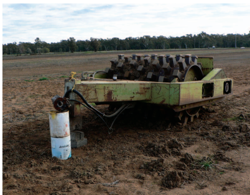
Sheepsfoot rollers are a popular piece of machinery for effective compaction.
