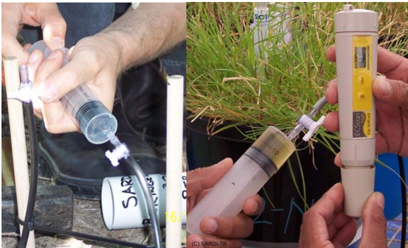
Figure 7. Using suction cups to extract soil water and measure soil salinity.
