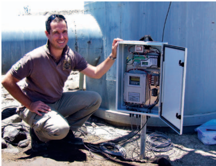
NCEA researchers Gary Sandell and Phil Szabo (pictured) are trialling a pump performance monitor they have developed, to provide data which will be used to examine pump efficiency.
