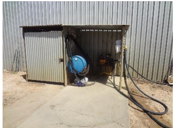
Wash down pad for cleaning machinery
