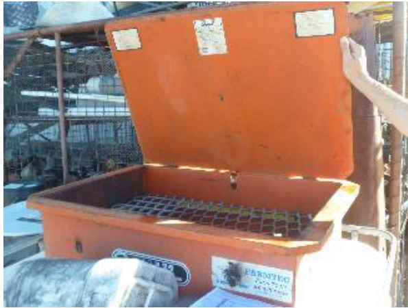
Waste oil management. Good area for draining oil filters
