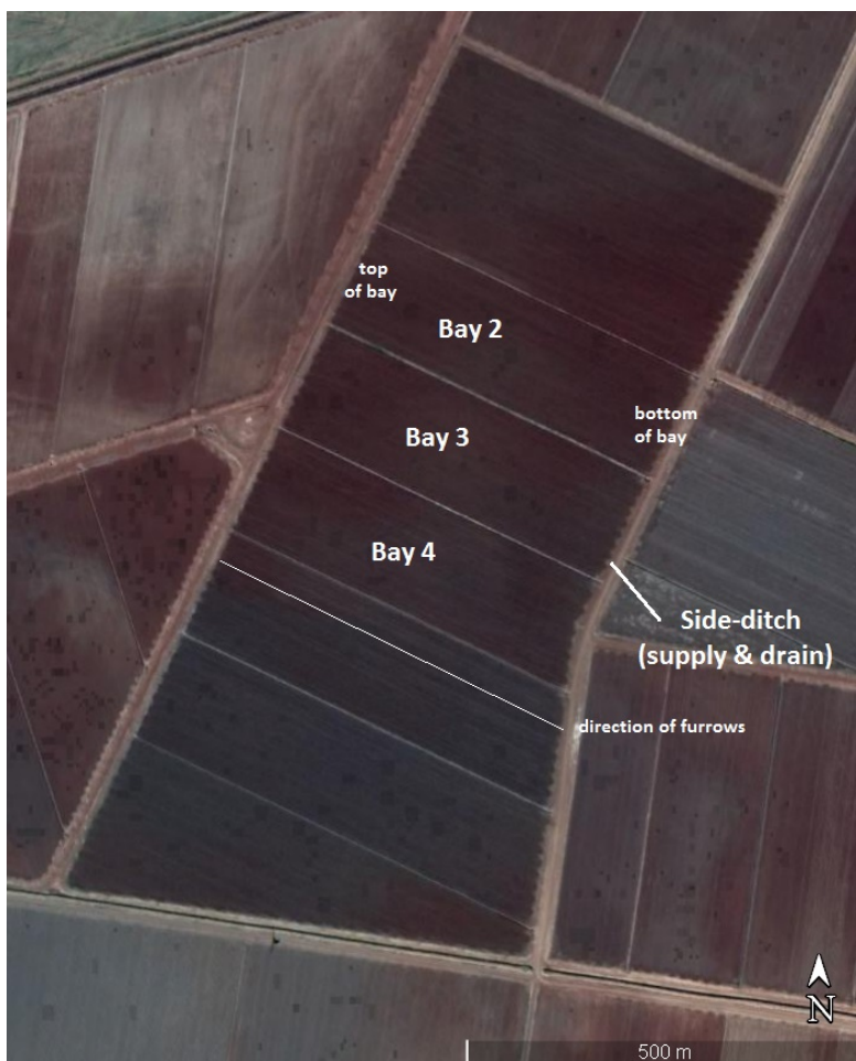
Figure 13: Aerial image of the level furrow system without laterals at Whitton (Field 7) used for collecting irrigation field data. The labels indicate the bays from which irrigation data was collected. The locations of key features (side-ditch; furrows) are also indicated. Scale and direction are shown.
