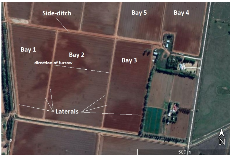
Figure 12: Aerial image of the level furrow system with laterals at Whitton (Field 19) used for collecting irrigation field data. Irrigation data was collected from bays 1, 2 and 3. The locations of key features (channels, furrow orientation) are also indicated. Scale and direction are shown bottom right.
