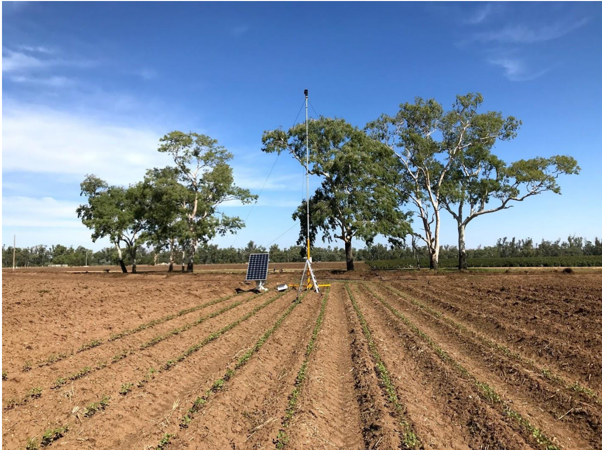
Figure 2: Thermal camera on a tower taking images to monitor crop stress during early cotton season at ACRI.
