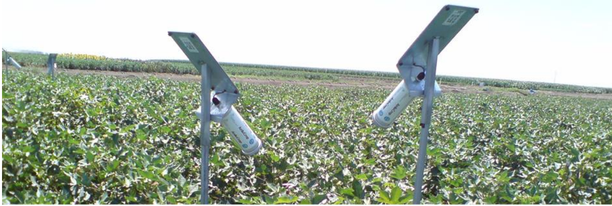
Figure 3: Canopy temperature sensors installed in a cotton field at ACRI
