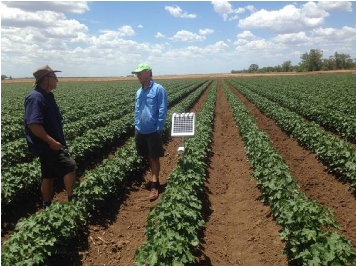
Figure 7: Canopy temperature sensor installed at a cotton farm in St. George, Queensland
