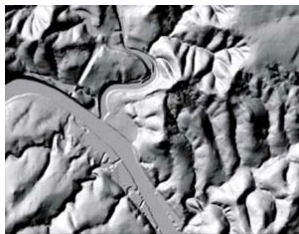
Figure 3-7 Digital elevation model DEM, (raster data)
