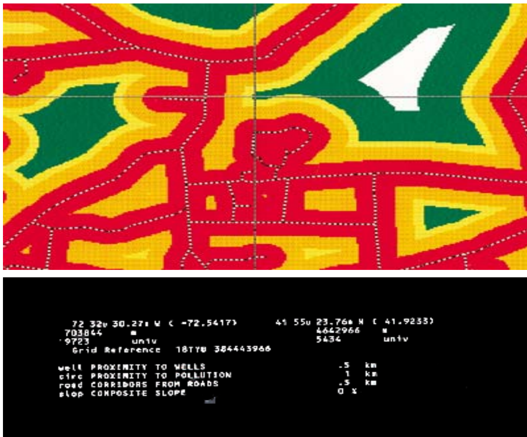
Figure 3–26 The cursor can be used to point to a location stored in an SIS and return attributes about the location such as longitude, latitude, soil type and slope
