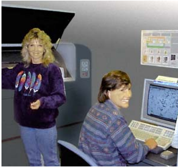
Figure 3–15 Scanning paper maps to produce digital data files for input into an SIS
