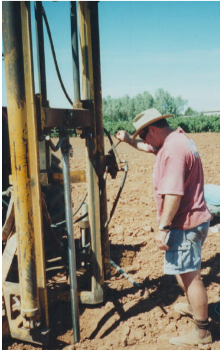
Figure 5-4. Hydraulic coring machine used to install EnviroScan installation tubes and take soil cores
