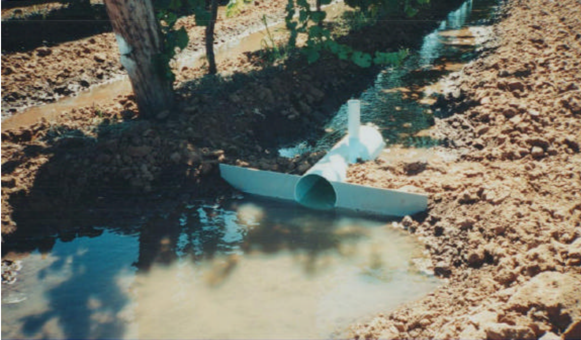
Figure 5-2. Front view of modified circular flume showing cut-off barrier used to prevent preferential flow around the sides of the flume
