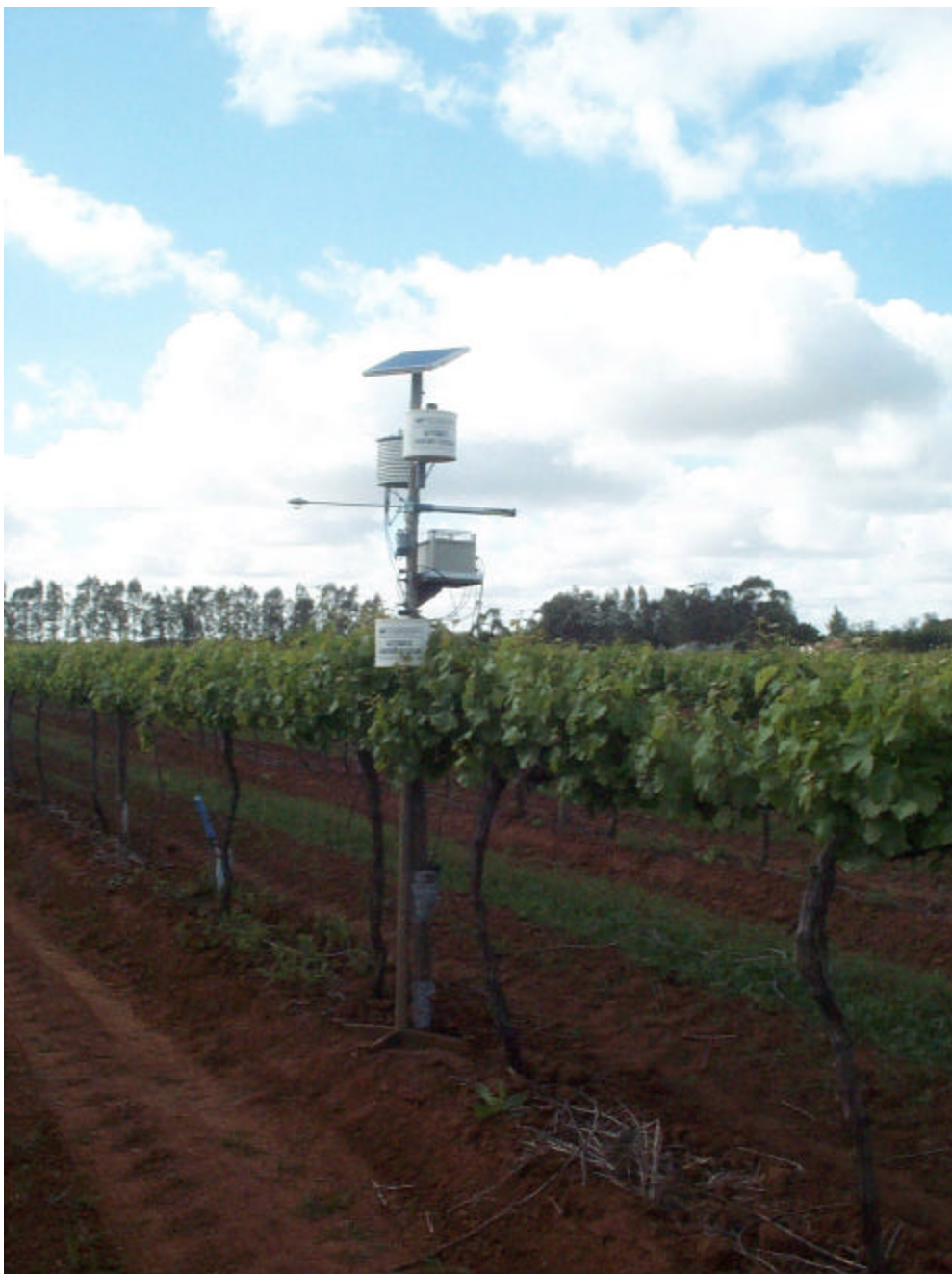
Figure 5-7. DREAM instrumentation used to measure evapotranspiration at the CWM site
