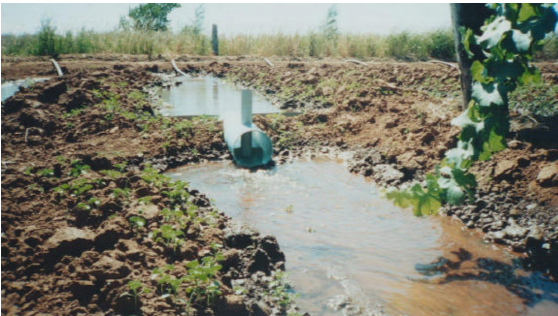
Figure 5-3. Rear view of circular flume showing positioning of flume in furrow and hydraulic jump during an irrigation event
