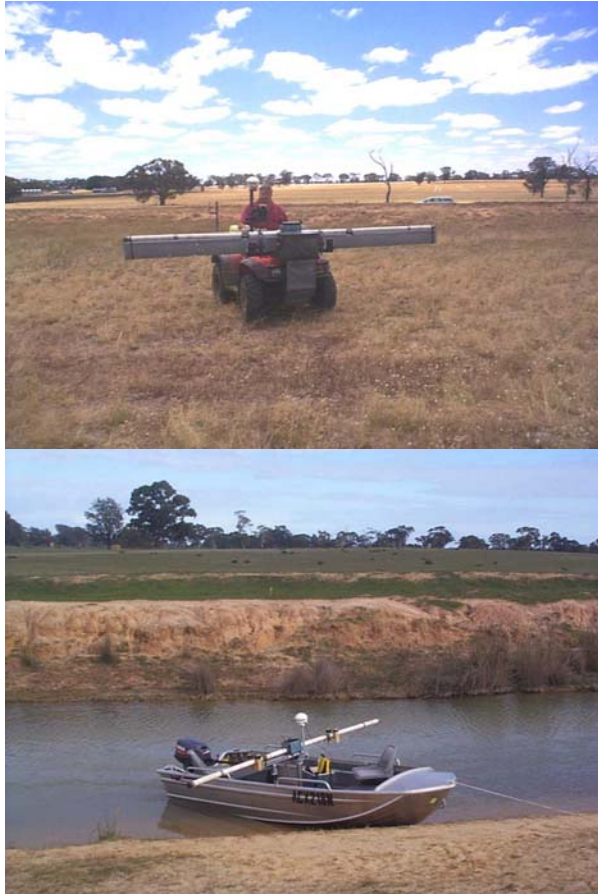
■ Figure 5.14 EM31 Set-up on Land and On-channel (Toolondo Channel August 2002)
