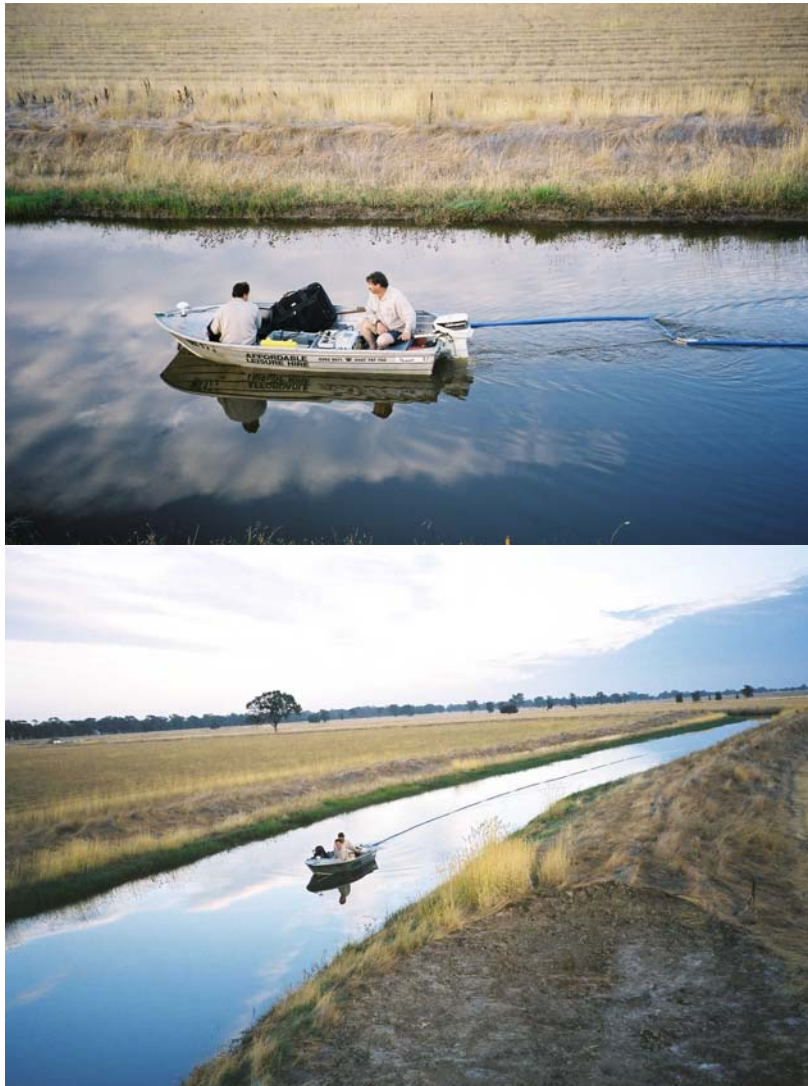
■ Figure 5.67 Resistivity Array Deployed in Year 3 Trials (in operation at the Toolondo East site)
