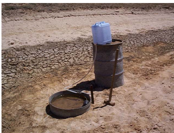
■ Figure 4-8 Ring Infiltrometer (left) and Disc Permeameter (right) in use at the Toolondo Channel
