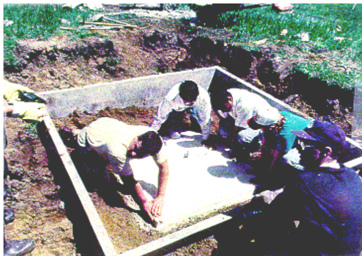
Figure 4.7: Installation of Double Ring Infiltrometer
