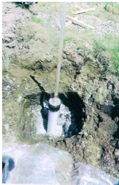
Figure 4.9: Two-stage Borehole Permeameter in Field
