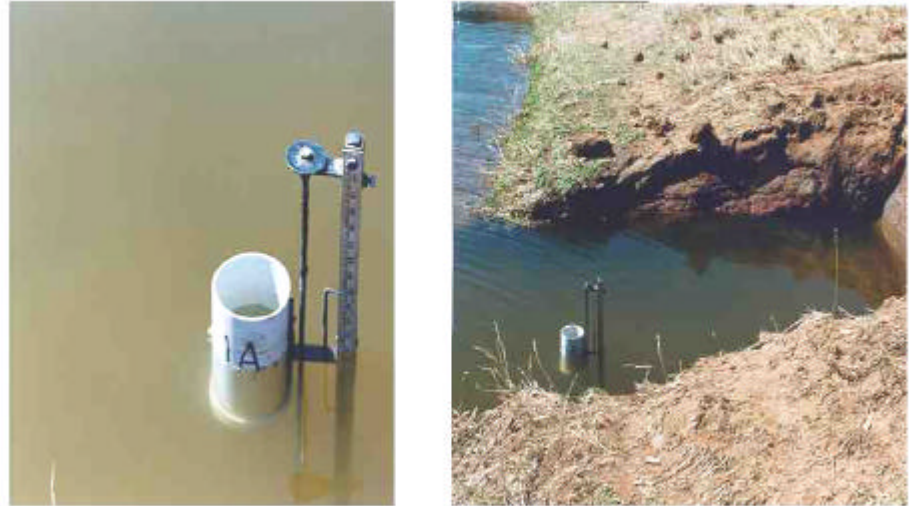
Figure 3.3: Hook Gauge Used For Measuring Pondage Water Levels
