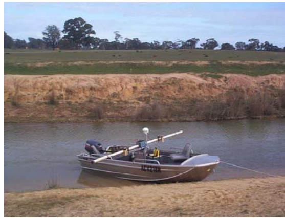
■ Figure 4-3 EM31 Mounted on Quad Bike and on Boat
