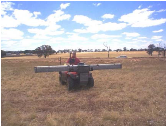
■ Figure 4-3 EM31 Mounted on Quad Bike and on Boat
