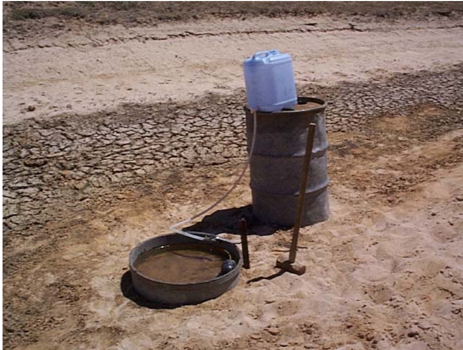
■ Figure 2-8 Ring Infiltrometer In Use In Dry Channel
