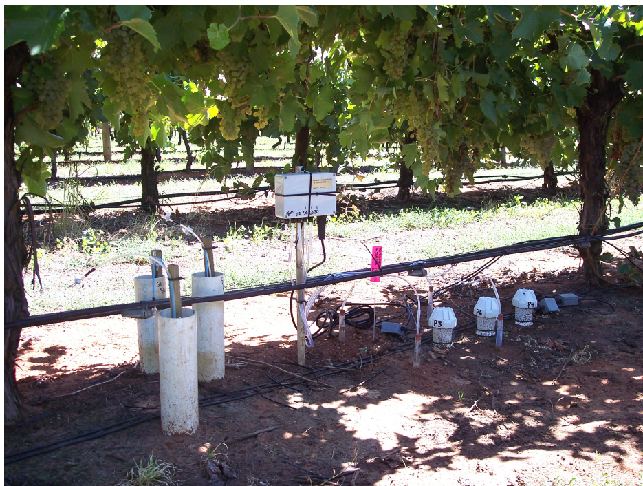
Figure 3. A fully instrumented drip irrigated vineyard at the Loxton Research Centre in the Riverland. Instruments in the picture include; capacitance probes, tensiometers, gypsum blocks, soil solution extractors, full and long stops
