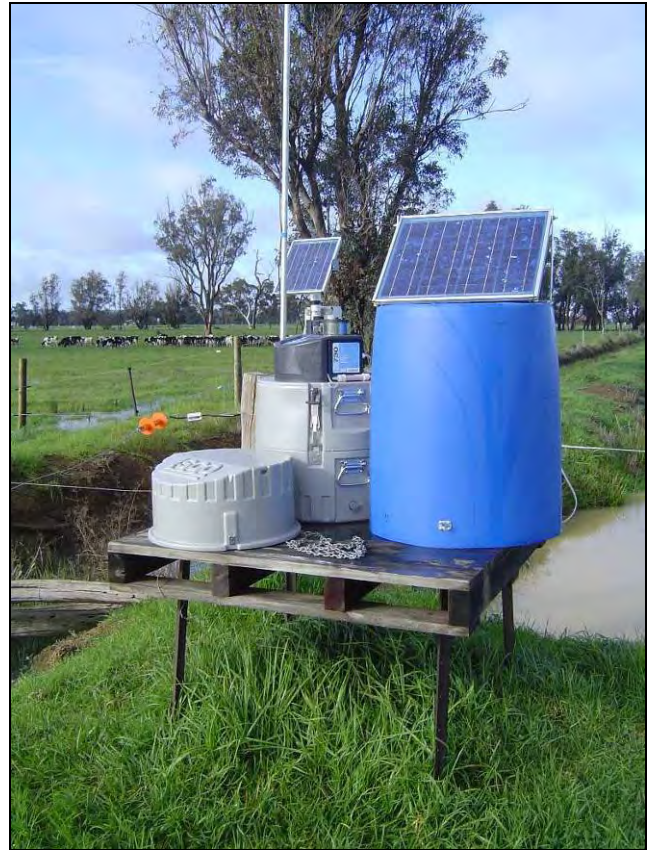
Figure 7: ISCO 6712 Automatic water sampler
