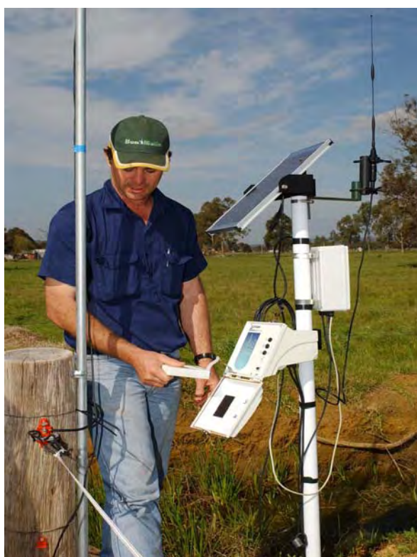
Dale checking soil moisture monitoring equipment (Arthur Mostead)
