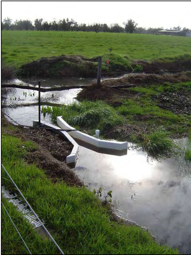
Figure 6: 6" Parshall Flume installed at Sit
