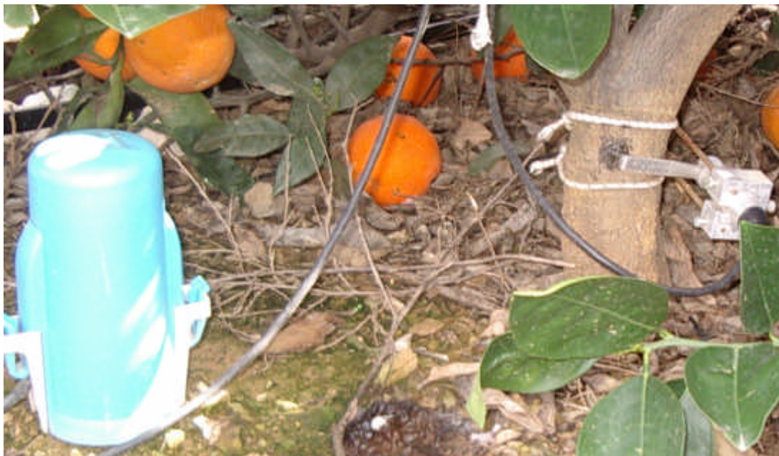
Figure 11: Soil capacitance probe (left) and a trunk diameter measuring device (right) used by a grower in Spain to assist in irrigation scheduling.
