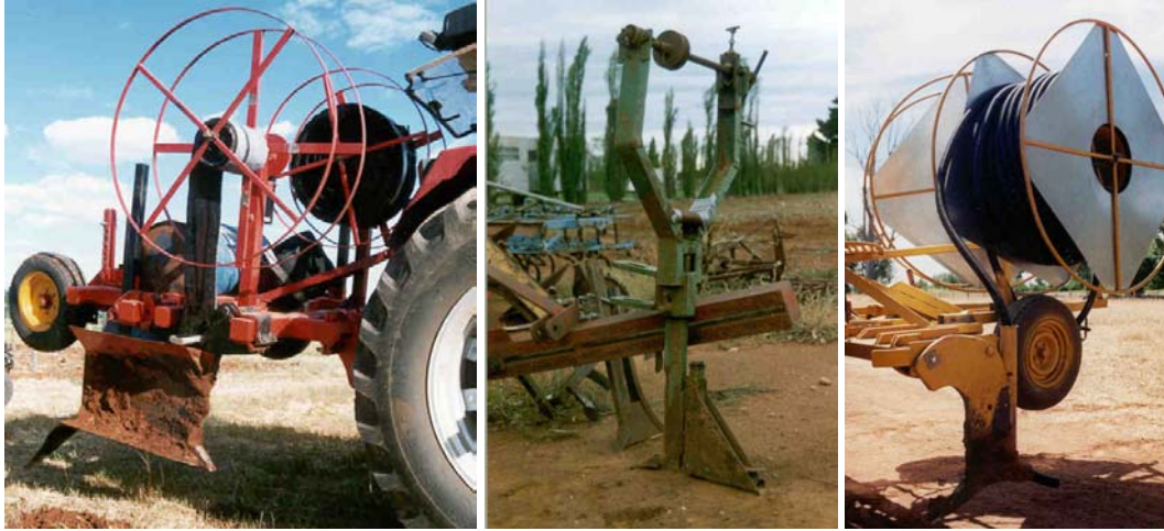
Figure 3.6. Buried irrigation pipe insertion machinery. CRZI (left), Drip Tape (middle), SIP (right).
