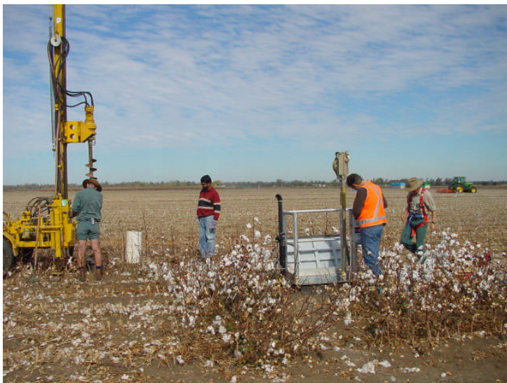
Figure 4 On the left - Grant Millar and (NR&M) installing one of the NR&M barrel lysimeters - close to (on the right) the large (shelve-type) CSIRO lysimeter at ACRI, Narrabri (May 2005). Picture courtesy of Dr. Des McGarry.
