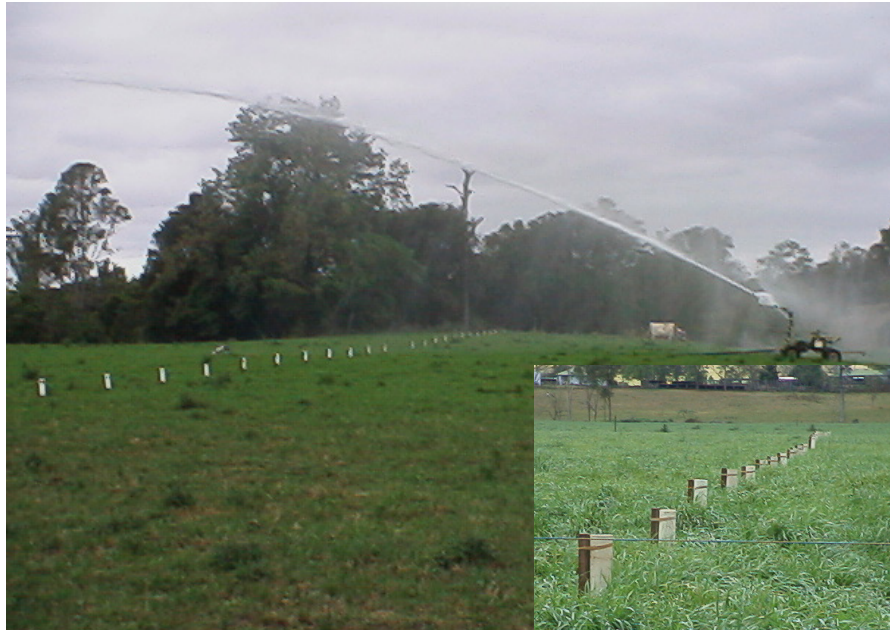
Figure 5. Catch cans laid out under a travelling gun irrigator to record the depth of water applied for use in calculating application uniformity (Table 8).
