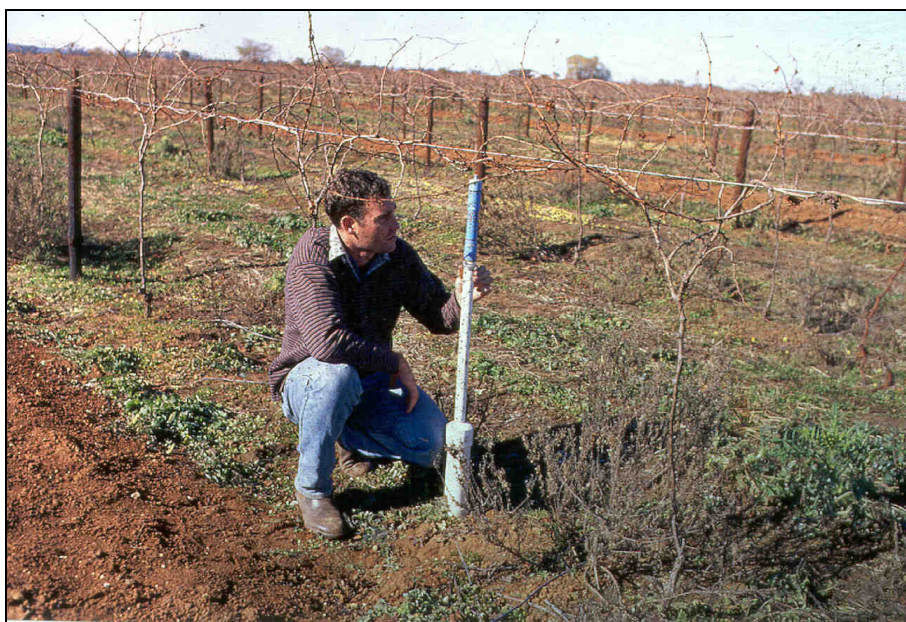
Figure 11. Testwell in vineyard with capacitance logger
