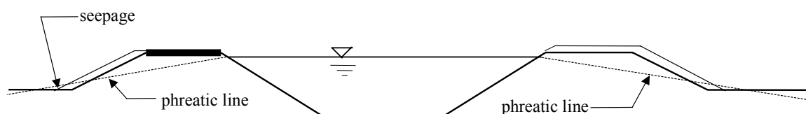
Figure 10.3 Phreatic line breached causing seepage
