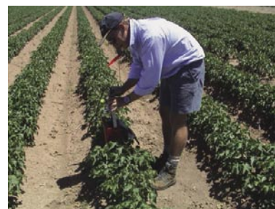
Using a neutron probe to measure soil moisture.
