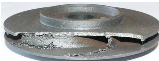
Cavitation damage to an impeller.
