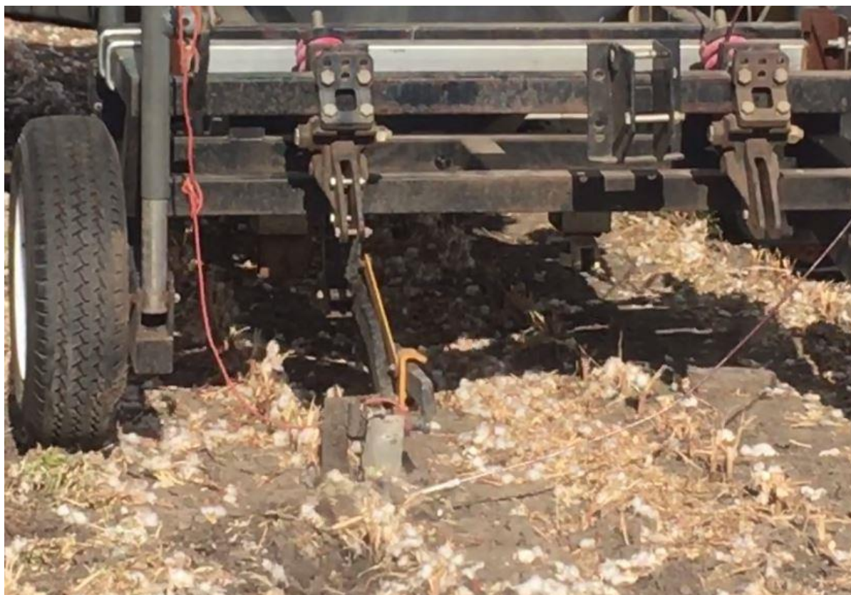
Photo 1. Shows the sheet metal engagement tool which held the AquaTill nozzle in place and funnelled the plant stems through for controlled contact with the cutting jet.
