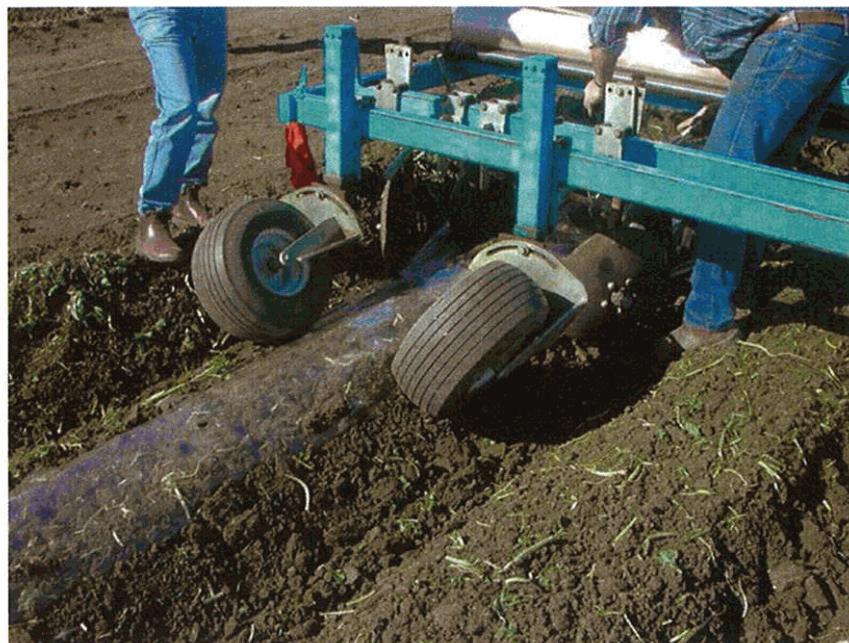
Figure 4.5. Covering beds with polythene film after incorporation of a green manure crop of mustard at the Australian Cotton Research Institute on 4 Sep 2003
