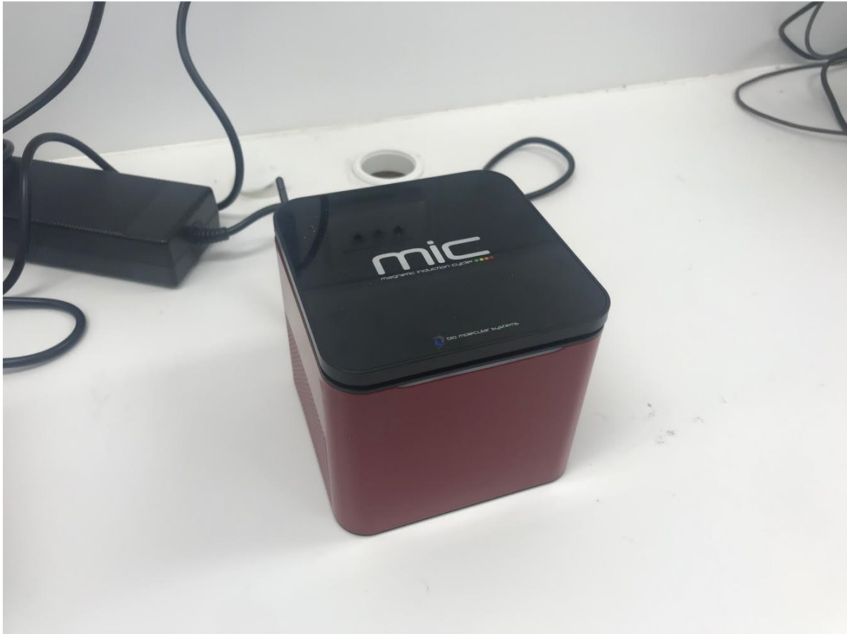
Figure 4.3.1. Micro 'MIC' qPCR machine sitting on a bench at the EMAI before being filled with spider mites for identification.
