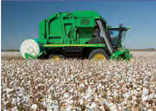
FIGURE 2: John Deere 7760 round module pickers have almost entirely replaced the more traditional picking machinery, allowing a more manageable and safer approach, with less casual labour. Growers utilising these pickers should consider, soil compaction and round module handling. (Photo courtesy of John Deere)
