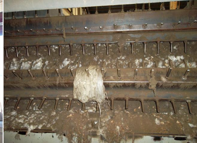
The photo above left shows the contamination sensors (the black boxes) developed by CSIRO and the Australian ginning industry mounted to the rear of the module feeder. The sensor alerts ginners when module wrap plastic is caught around the beaters in the feeder (above right).
