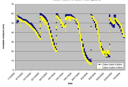
**Figure 3**. Water extraction from continuous cotton and cotton vetch rotation showing slightly higher water holding capacity of soils after vetch.
