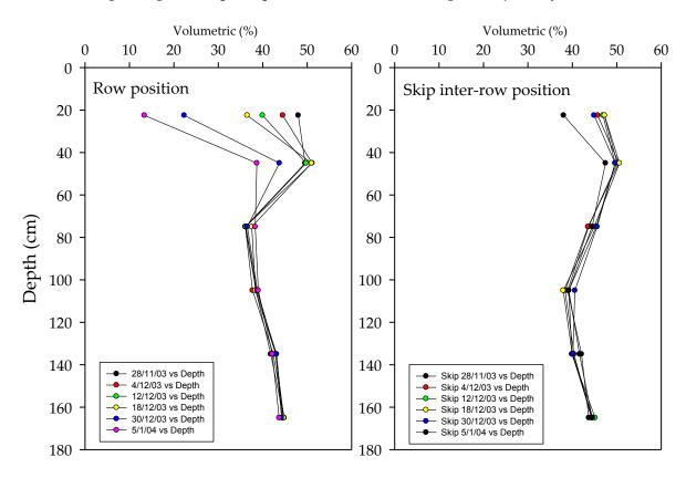
**Figure 1.** Water extraction for various dates in skip row cotton, with measurement take from neutron probes in the plant line (row position) or in the skip row (skip inter-row position. There was little extraction from the skip area.
