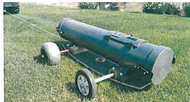
A homemade buggy is used to tow an EM38 behind a Quad bike over irrigated dairy paddocks in Victoria. (Buggy and Photo provided by Stewart Spillsbury)
