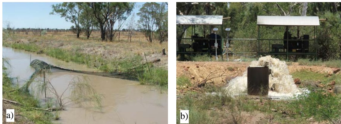
Fig. 6.3: a) Fyke net set up for sampling pumped water at Jericho PS, b) pump station showing the first water coming through the outlet pipe.
