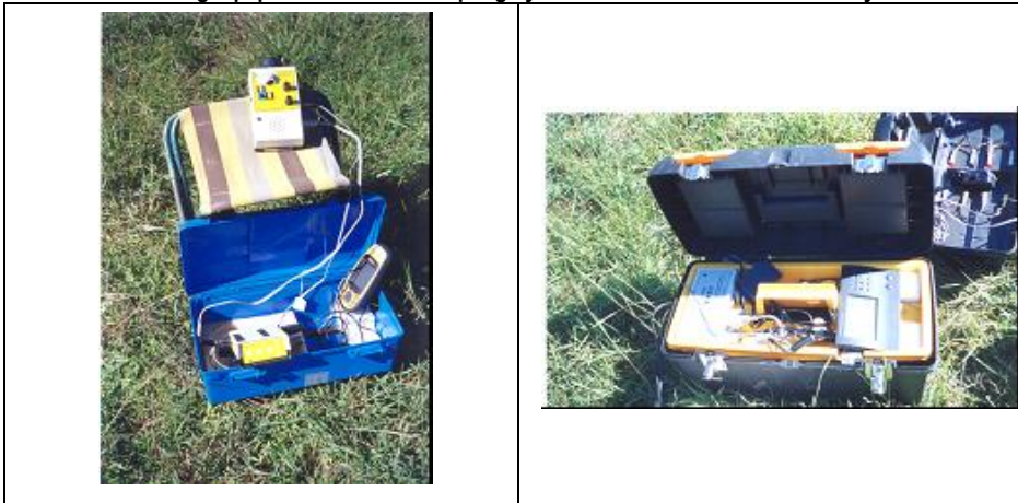
Plate 4.3.a. Anabat II bat recorder and CF Storage ZCA Interface Module (Tittle Electronics Pty. Ltd.) and Magellan Meridian GPS
