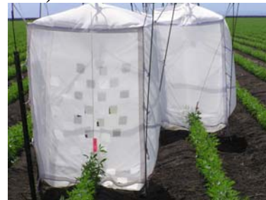
(c) Open tents could be effectively closed by securing a window (100 x 200cm) to the Velcro on the edge of the holed face of the tent.
