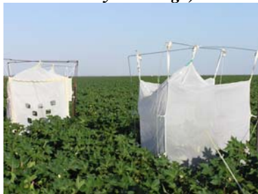
(a) The tents were secured by elastic to a steel frame that was positioned over it and pegged into the ground.
